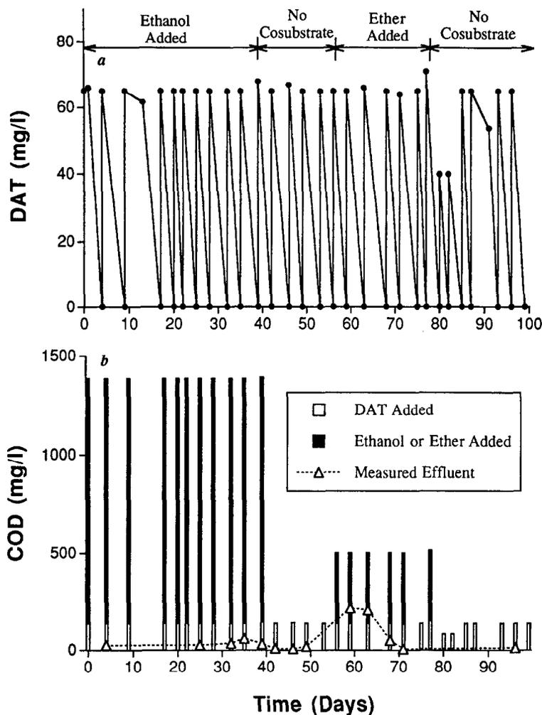
Fig. 1. Biodegradation of DAT, showing (a) repetitive additions, with and without ethanol and ether added; and (b) COD contributed by DAT plus ethanol or ether, and soluble COD in effluent samples. Results shown are for one bottle of a pair; the behavior of the duplicate was very similar.
