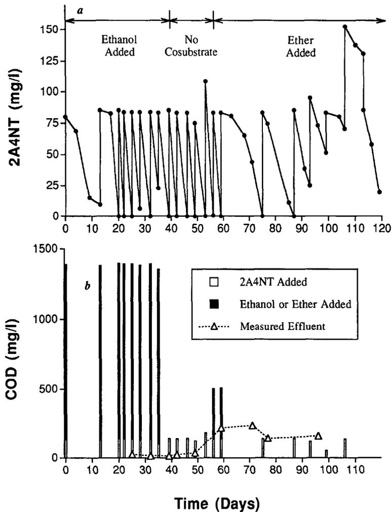
Fig. 3. Biodegradation of 2A4NT, showing (a) repetitive additions, with and without ethanol and ether added; and (b) COD contributed by 2A4NT plus ethanol or ether, and soluble COD in effluent samples. Results shown are for one bottle of a pair; the behavior of the duplicate was very similar.
