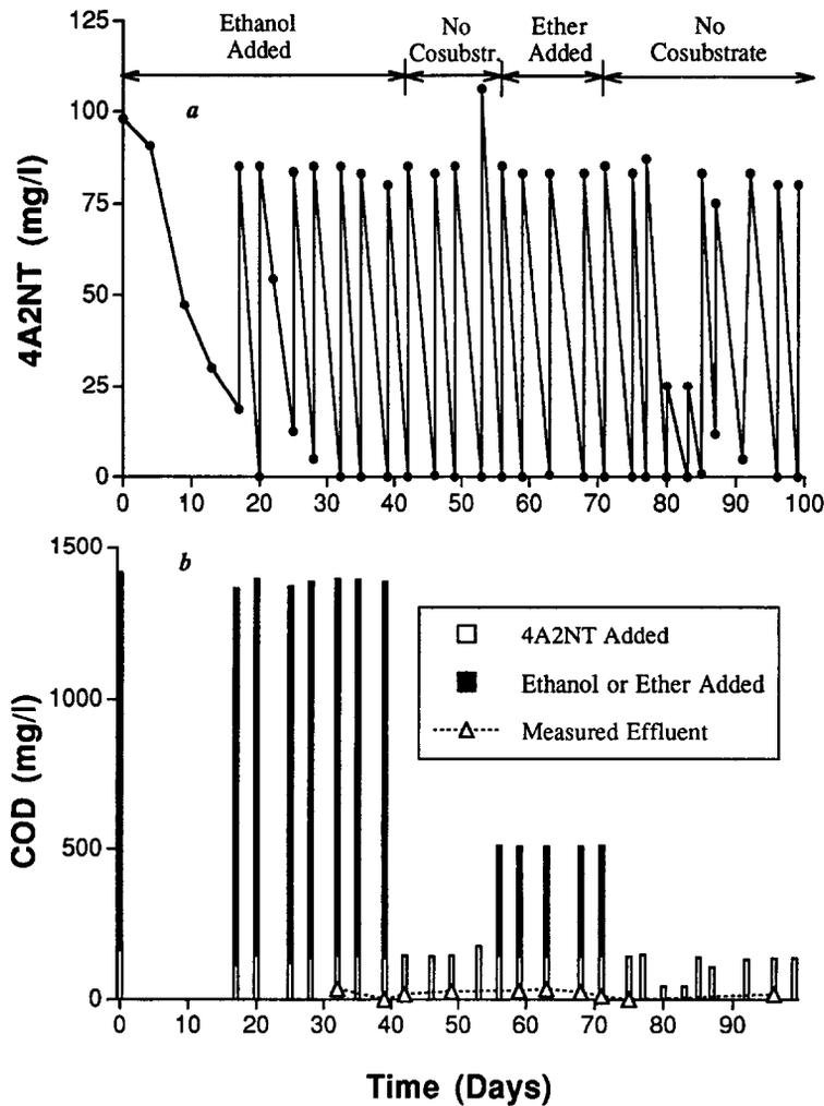
Fig. 2. Biodegradation of 4A2NT, showing (a) repetitive additions, with and without ethanol and ether added; (b) COD contributed by 4A2NT plus ethanol or ether, and soluble COD in effluent samples. Results shown are for one bottle of a pair; the behavior of the duplicate was very similar.
