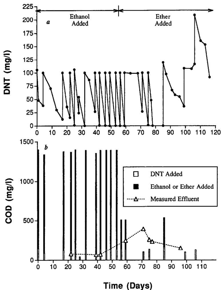
Fig. 4. Biodegradation of DNT, showing (a) repetitive additions, with ethanol or ether added; and (b) COD contributed by DNT plus ethanol or ether, and soluble COD in effluent samples. Results shown are for one bottle of a pair; the behavior of the duplicate was very similar.
